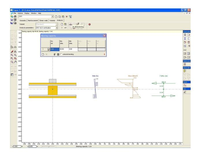
FAGUS-5W is an optional module of your familiar FAGUS-5 that allows the design of wooden cross-sections. The particularity of this material is the intense orthotropic properties that have to be taken into account.
